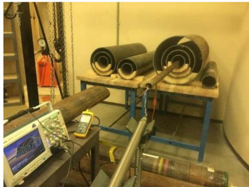
Figure 8a—Lab setup of four pipes nested concentrically
